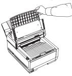
2. Press in the cover release buttons on the sides of the copy stacker until you hear a click. Lift the copy stacker.
